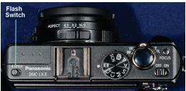
The flash switch is on top of the camera at the far left. It has only one function -- to unlatch the flash mechanism so it can pop up and be available in case conditions call for its use. If you, the user, do not manually pop the flash unit up using this switch, it will not be available, because the camera cannot pop the unit up automatically.
