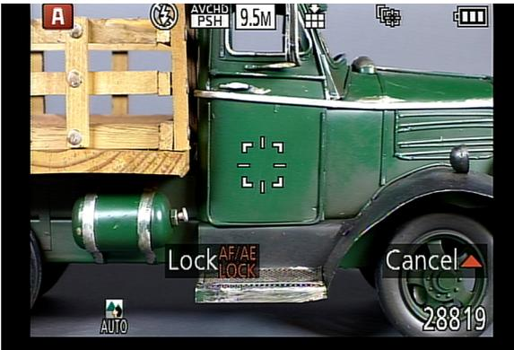
Fig. 3-13: AF Tracking Focus Frame on Screen
