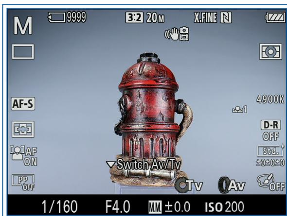
Figure 3-22. Display When Control Wheel Adjusts Shutter Speed
