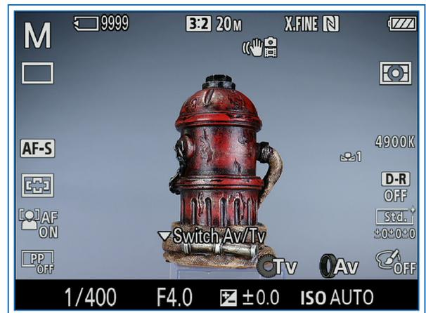
Figure 3-25. Manual Exposure Screen with Auto ISO in Effect
