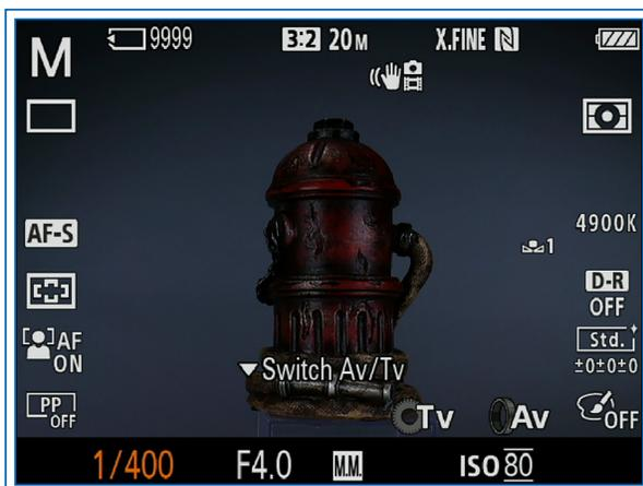
Figure 3-24. Manual Exposure Screen with Setting Effect On
