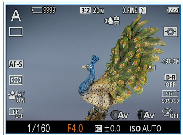
Figure 3-16. Aperture Setting from Using Control Wheel
