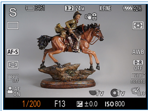
Figure 3-15. Shutter Speed Setting on Shooting Screen
