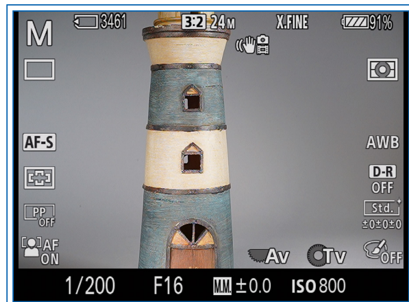
Figure 3-17. Aperture and Shutter Speed Values on Shooting Screen
