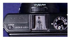
The flash switch is on top of the camera at the far left. It has only one function -- to unlatch the flash mechanism so it can pop up and be available in case conditions call for its use. If you, the user, do not manually pop the flash unit up using this switch, it will not be available, because the camera cannot pop the unit up automatically.
