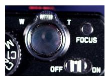
This control is quite familiar by now. You press it down halfway to check focus and exposure, and press it the rest of the way to record the image. You can also press it to wake the camera up from Power-Save mode. The shutter button has a somewhat different use when you are making multiple exposures using that option on the Recording menu. After the initial exposure is made, you move to the next one by pressing the shutter button halfway down.
