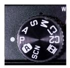
The Mode dial is on top of the camera to the right of the hot shoe as you hold the camera in shooting position. We discussed this dial extensively in Chapter 4. Its settings move you between the various modes of shooting: Snapshot, Program, Aperture Priority, Shutter Priority, Manual, Custom 1, Custom 2, Motion Picture., and Scene. If you happen to leave the Mode dial in a position that does not select one of those set-
