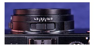
This switch, located on top of the lens barrel, has three possible settings: 4:3, 3:2, and 16:9, representing the ratio of the width of a horizontal image to its vertical height. This setting does not affect just the shape of the image; it also determines how many megapixels an image can contain. When the aspect
