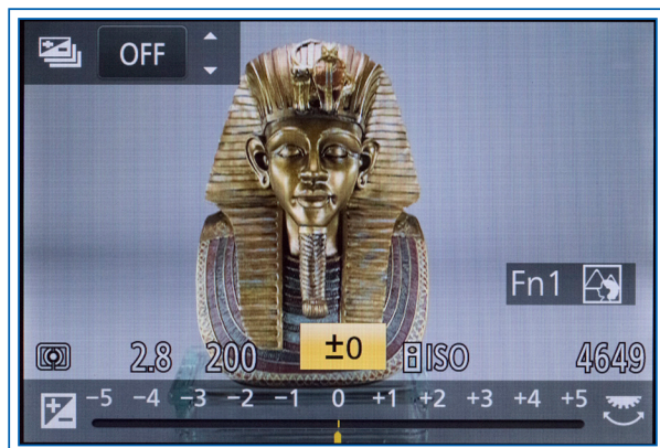
Figure 3-9. Exposure Compensation Scale on Display
