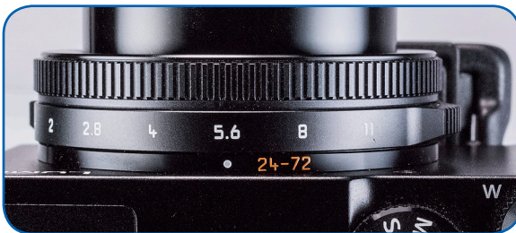
Figure 3-22. Aperture Ring at f/5.6
