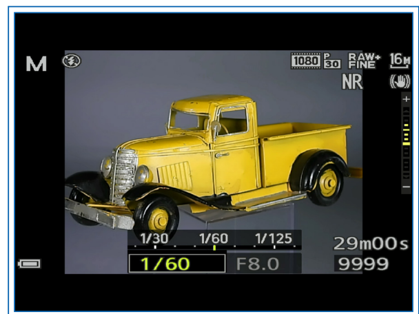
Figure 3-17. Tick Marks Indicating Overexposure
