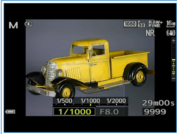
Figure 3-18. Tick Marks and Triangle Indicating Underexposure
